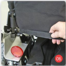
The angle of the backrest of your electric wheelchair has a manual recline function and can be easily adjusted to the wanted position by pulling the strap at the lower end of the backrest. You also have the option of folding the backrest completely down to the front.
