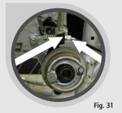
is set using the adjusting screw (Fig. 31). The braking power is increased by unscrewing the adjusting screw and reduced by tightening it.
